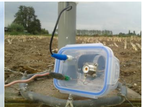
Matchbox of our 15m antenna, this one just needed an inductor to get the right impedance.
