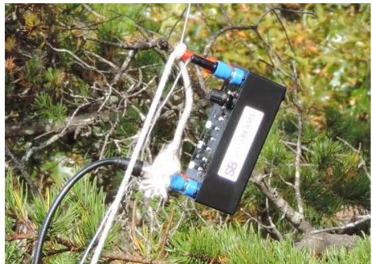
The 80-10m adventure-tuner (a kit from SOTABEAMS), hanging from the end-fed inverted-L.
